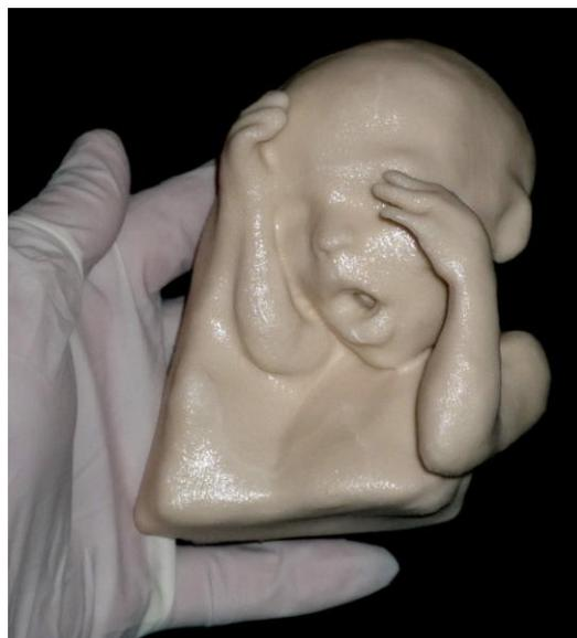
Figure 13- Final Rapid prototype model, exhibiting both arms, built on Z-Corp equipment at LAMOT- Laboratory, Instituto Nacional de Tecnologia - Rio de Janeiro, Brazil
