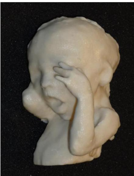
Figure 10- First Rapid prototype model, exhibiting only the left arm, built on Z-Corp equipment at LAMOT- Laboratory, Instituto Nacional de Tecnologia - Rio de Janeiro, Brazil.
