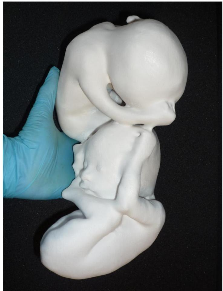
Figures 6 and 7- Rapid prototype models of fetuses built on Z- Corp equipment at Rapid Form laboratory. Royal College of Art - London, UK.
